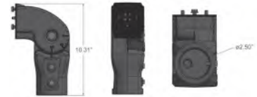
SF - Slip Fitter Arm Dimensions
