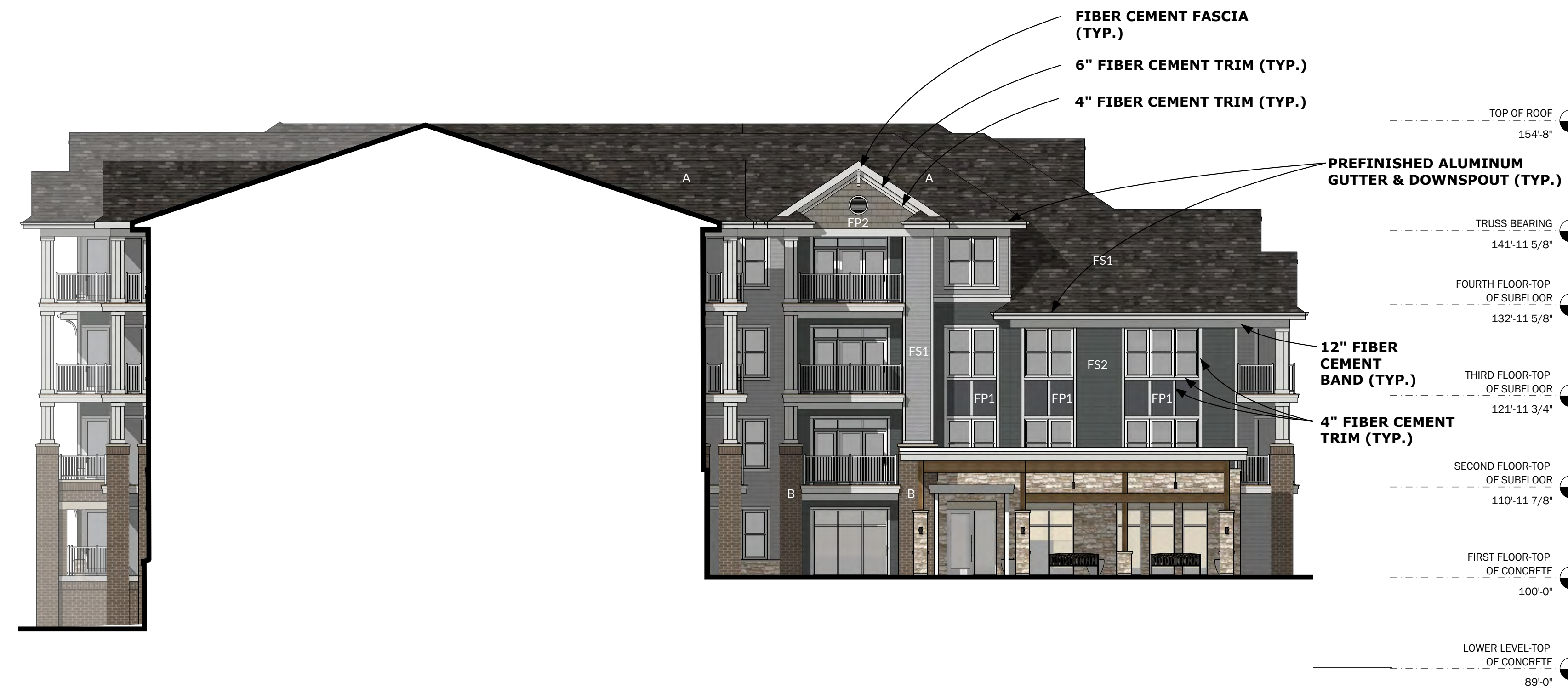
MAIN ENTRY | SOUTH ELEVATION
