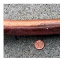
**Copper**. After scratching, if the pipe is the same color as a penny and may have a solid or splotchy film, varying in color from bright green to dark brown, you may have a copper pipe. A scratch test on copper pipe will expose a shiny copper penny color. If you place the magnet on the pipe and it does not stick, this confirms this is not copper.
